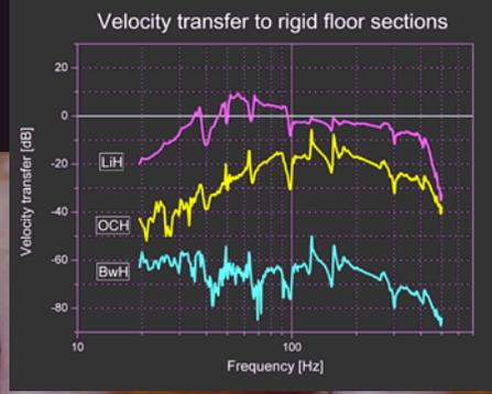
In BwH, the rigid floor sections are parquet glued onto bedrock. In OCH it is parquet glued onto concrete, while in LiH, parquet on joists, 30 cm apart, are resting on thin rubber blocks.
