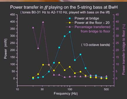
In the low register, the foundation has a noticeable impact on the bridge impedance, and thus the damping of the strings.
