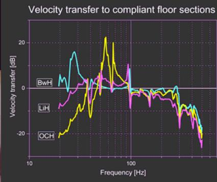
In BwH and OCH the compliant floor sections are stage lifts. Although preferred by the bassists, these give pronounced resonances.
