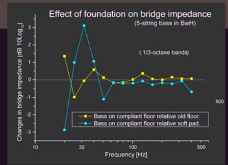
In BwH and OCH the stage lifts are the preferred areas for double basses. Contradictory to that, the BwH was originally constructed with the flooring glued with asphalt onto solid bedrock. After a few years with musicians complaining about "lack of dynamics", "insensitivity to tone-colour variations", "lack of warmth", and "lack of contact" the stage was reconstructed and the major part of the floor furnished with stage lifts.
