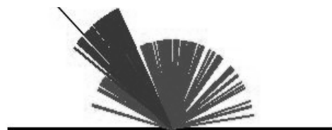
Fig.5: Scattered rays: left the single (long) specularly reflected ray, around that, for DG=25%, the scattered ray vectors (enlarged), the short rays are the cosine-type scattered rays of the first computation step.
