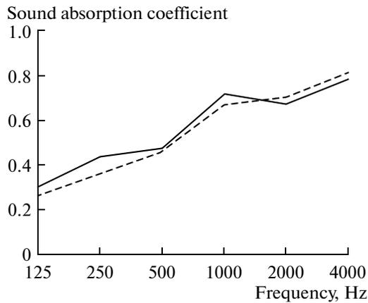
**Fig. 3.** Sound absorption coefficients of new (solid line) and original (dashed line) seats of chairs of the orchestra seating area.
