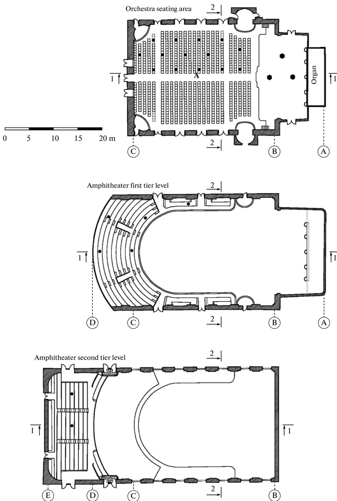
**Fig. 1.** Plans for Great Hall. Hexagons mark positions of the sound source on the stage, points indicate seats at which impulse responses were detected. The impulse response measured at point A is shown in Fig. 5.
