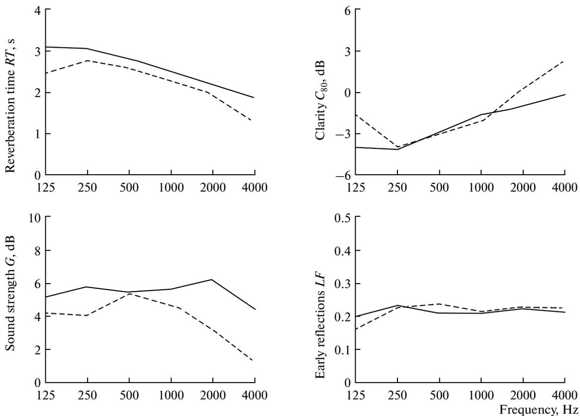
**Fig. 6.** Results of measurements of acoustic parameters of Great Hall after reconstruction (dotted line refers to measurements before reconstruction according to [4]).
