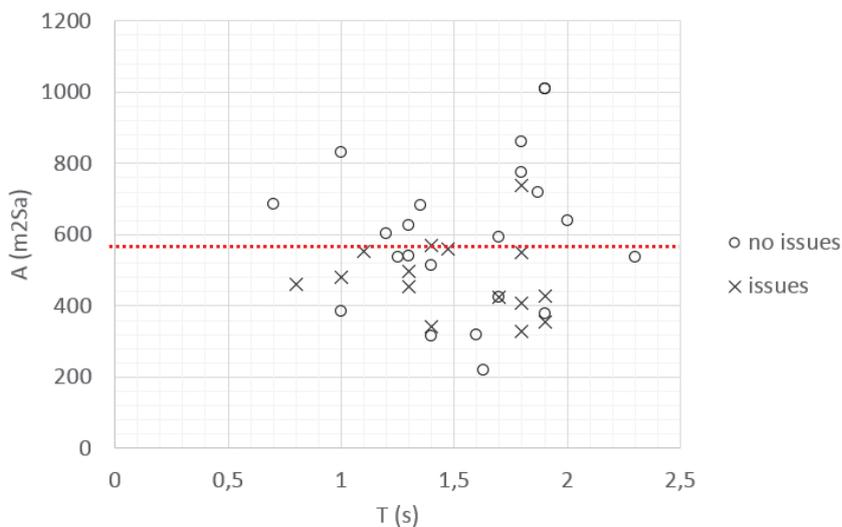
Figure 5 – Absorption area limit  $A=560\text{m}^2\text{Sa}$ , independent of  $T$
