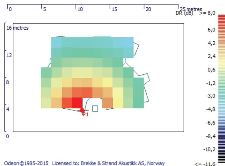
Figure 6 –  $D-R$  (dB) over orchestra in a 5000m<sup>3</sup> room, simulated in Odeon 14
