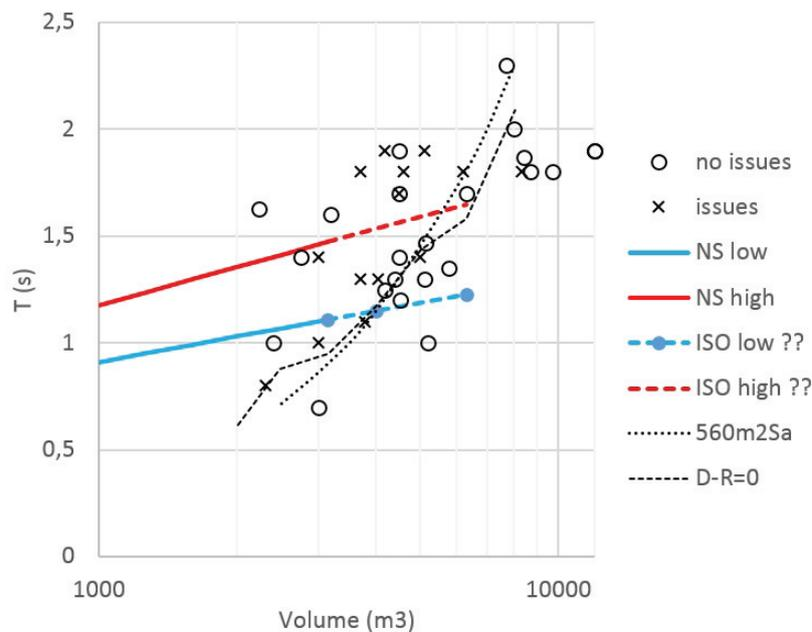
Figure 9 – plot of the data set  $N=37$ , NS-limits, possible extrapolations, “issues limit” ( $A=560\text{m}^2\text{Sa}$ ) and the limit corresponding to the criterion  $D-R=0\text{dB}$ .
