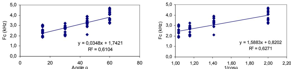
Figure 3. High pass filter cut off frequencies  $F_c$  plotted against incidence angles (left), and against projected element density  $1/\cos\theta$ , re 1 at normal incidence.
