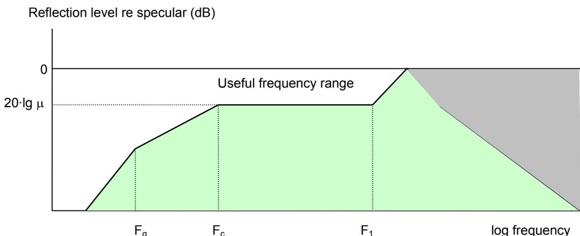
Figure 4: A summary of the flat panel array frequency limits.
