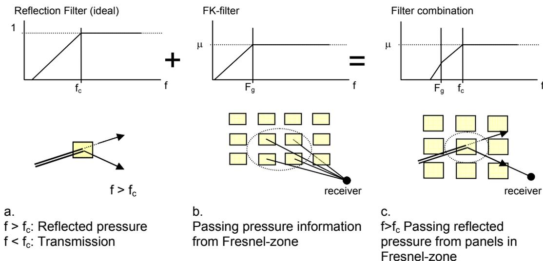
Figure 1. Frequency response as a serial combination of two filters
