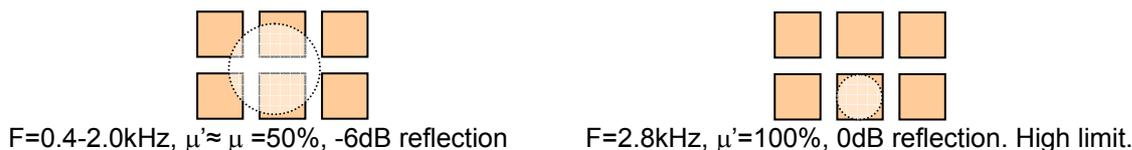
Figure 5. Useful frequency range depends on element size and shape related to Critical Zone
