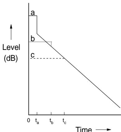
Figure 1. Integrated impulse curves at three receiver distances from a source in a room according to revised theory. Here,  $t = 0$  is the time when the sound was emitted from the source,  $t_a$  is the direct sound arrival time at position A close to the source. Positions B and C are progressively further from the source.
