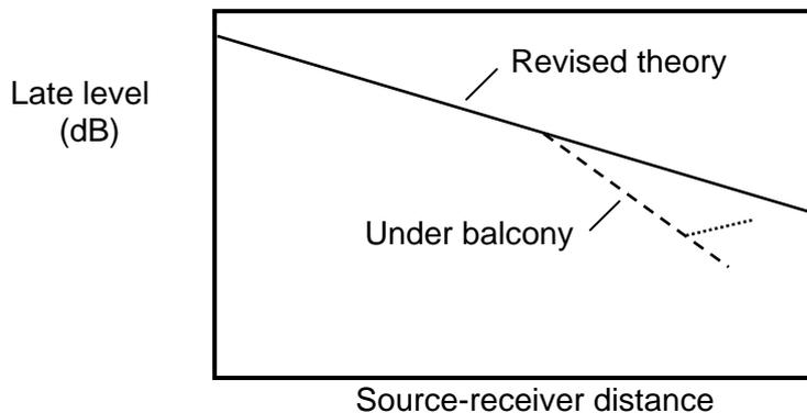
Figure 4. Simple model for behaviour of late sound under a balcony overhang (dashed line). The dotted line shows possible behaviour towards the rear of the overhang seats.
