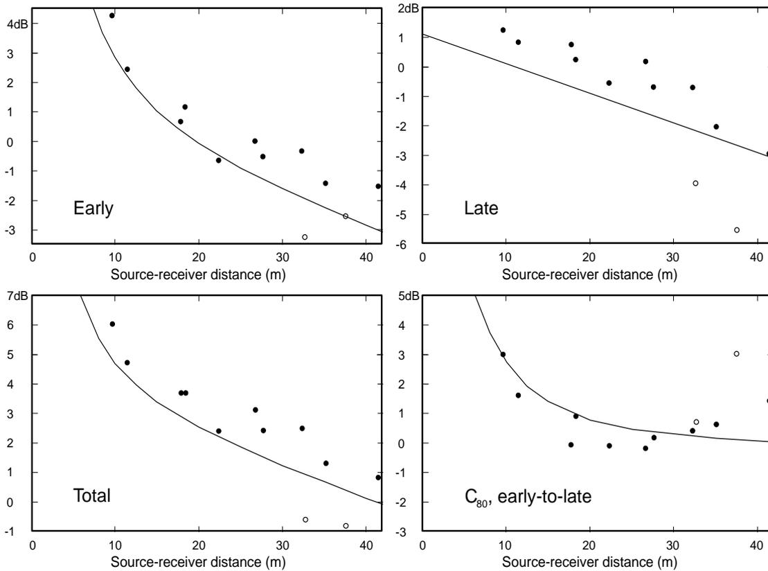
Figure 3. Values of early, late, total and C<sub>80</sub> levels in the unoccupied Royal Festival Hall, London, measured in 1982. Lines represent values according to revised theory. Open circles (o) represent measured values at seats below the balcony.
