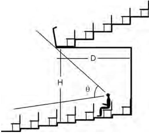
FIG. 1. Basic balcony overhang dimensions, showing the vertical angle of view,  $\theta$ .
