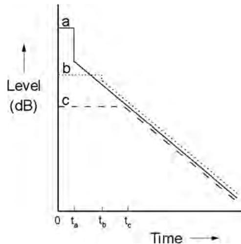
FIG. 2. Theoretical integrated impulse curves at three receiver distances from the source in a room. Curve “a” represents the position closest to the source, with travel time  $t_a$  for the direct sound. The time origin at  $t=0$  is the time when the sound is emitted from the source. According to assumption (1), the diagonal lines are superimposed but have been separated here for clarity.
