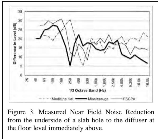
Figure 3. Measured Near Field Noise Reduction from the underside of a slab hole to the diffuser at the floor level immediately above.
