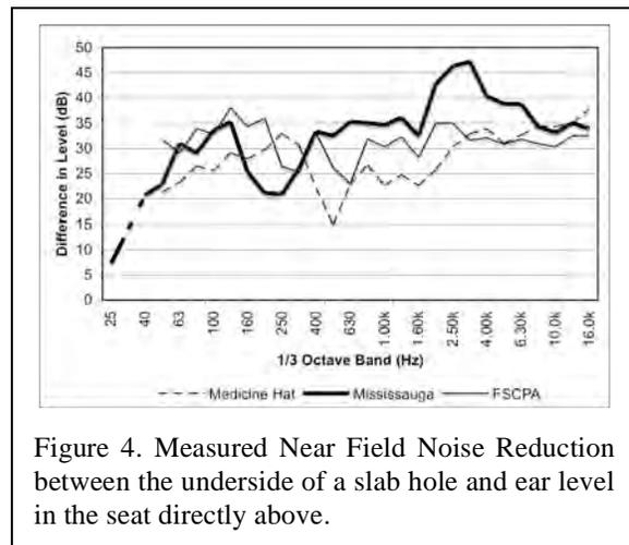
Figure 4. Measured Near Field Noise Reduction between the underside of a slab hole and ear level in the seat directly above.
