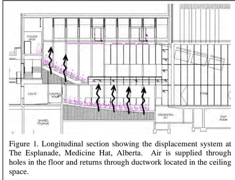
Figure 1. Longitudinal section showing the displacement system at The Esplanade, Medicine Hat, Alberta. Air is supplied through holes in the floor and returns through ductwork located in the ceiling space.
