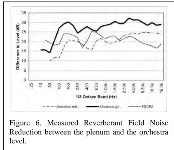
Figure 6. Measured Reverberant Field Noise Reduction between the plenum and the orchestra level.
