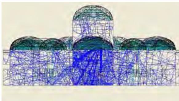
Figure 5: Propagation of rays from source 1
