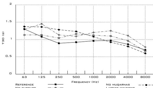
Figure 6: Simulated T30 in 4 different configurations
