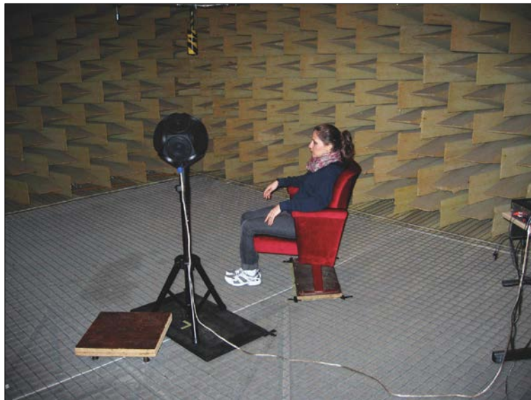
Figure 4.3. Laboratory experiments of masking thresholds, including the directivity characteristics – view from position of the loudspeaker 2 (Trumpet). The experiments were carried out in the anechoic chamber of the Division of Applied Acoustics of Chalmers University of Technology. (Photo by Behzad Ranjbari)
