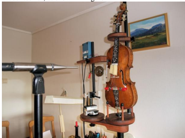
Figure 1: Rig for measurement of SPL(\omega)/F(\omega) "impact hammer" spectra. The fiddle is insulated from the rig by rubber bands. The strings are damped with rubber foam pieces.
