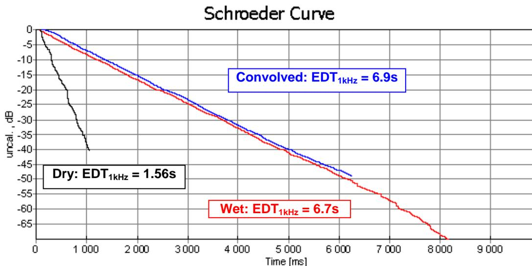
**Figure 6: Example of a ‘wet’ IR here working as ‘dry’ (from the stalls in Scene II), a wet IR from Tomba Emanuelle (red), and the resulting convolved IR (blue)**
