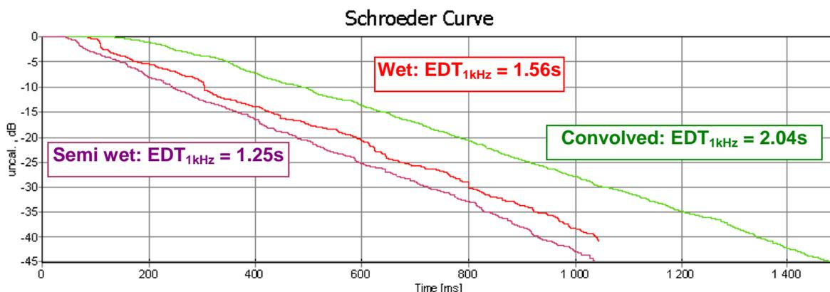
Figure 4: Example of a semi wet IR convolved with a wet IR. Examples are calculated impulse responses from the Scene II. P2 (dark red, semi wet), S1R3 (red, wet) and P2 convolved with S1R3 (green).
