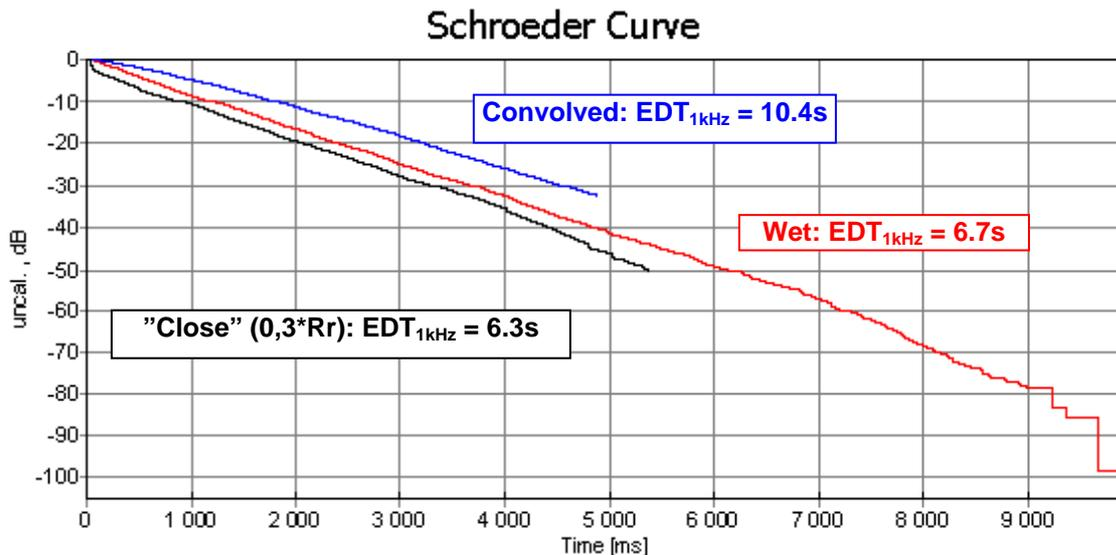
Figure 5: Example of a close ( $d=0.3 \cdot R_r$ ) recorded IR (black) convolved with a wet IR (red) making the convolved (blue) IR.
