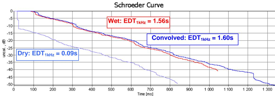
Figure 3: Example of a “dry recording” convolved with a “wet” one. S1\_1m (light blue, dry), S1R3 (red, wet) and S1\_1m convolved with S1R3 (blue).
