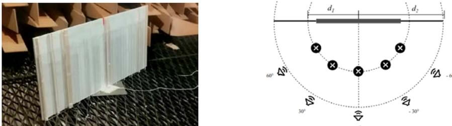
Figure 3: (Left) Picture of the scattering measurement of the broadband metadiffuser; (Right) Diagram of the measurement layout displaying source (S) and receiver (R) positions around the test surface at specific angular positions from the geometric centre of the surface, where  $d_1$  and  $d_2$  are 1.5 m and 3 m, respectively.
