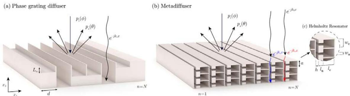
Figure 1: (a) Scheme of a QRD Schroeder diffuser composed by  $N = 7$  wells or quarter wavelength resonators. (b) Metadiffuser composed of  $N = 7$  subwavelength slits, each of them loaded by  $M = 3$  Helmholtz resonators. (c) Detail of a slit of the metadiffuser showing the geometrical parameters of the cavity of a HR ( $w_c$  and  $l_c$ ) and its neck ( $w_n$  and  $l_n$ ). (After Jimenez et al.<sup>14</sup>)
