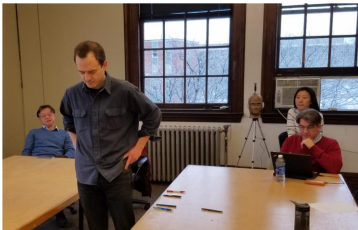
Figure 4: Finding the LLD in a small lecture room at Rensselaer University. Subjects put a pencil on the table where they could no longer localize two speakers in front playing separate anechoic violin parts. The room was small and reverberant. The dummy head and the 3D microphone used in the measurements can be seen in the background.
