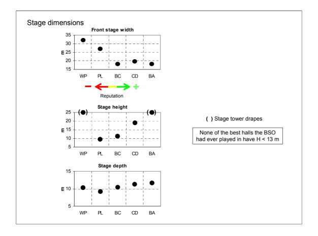
Based on the observation of the positive effects of narrow side walls and high ceiling, it is interesting to study the significance of stage width, height and depth. The width is measured on stage front where the strings are sitting. When looking at the front stage width related to reputation, narrow stages are preferred, while greater height is preferred. The heights in Weymouth and Basingstoke are not so relevant because they have an absorbing stage tower.
