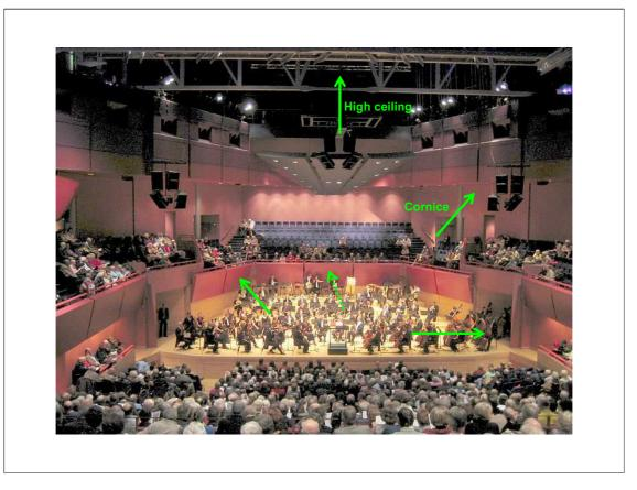
If we take a look at the stage in Basingstoke we can recognise many of these positive elements for a good level balance: High ceiling, narrow stage, tilted reflecting panels along the edge of the stage and cornice reflection from the side. The effect of the rather small reflector in this hall, tilted to reflect down towards the audience at the stalls, has not been properly investigated yet.
