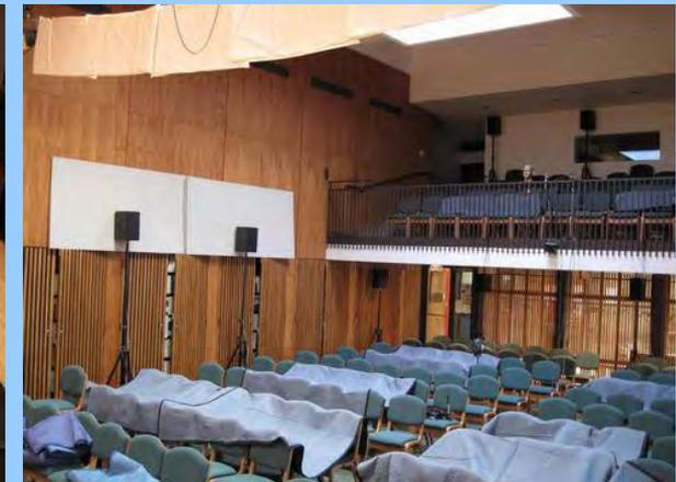
The absorptive curtains at the rear of the stage could be rapidly withdrawn. The blankets that simulated audience could be removed in 5 minutes, along with the panels on stage. This allowed prompt A/B comparisons. Some of the 25 LARES enhancement speakers are visible
