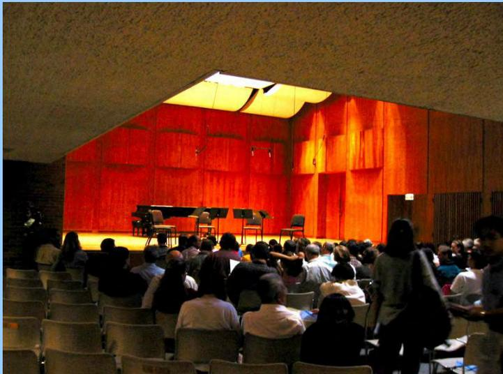
Note the highly reflective stage and side walls, deeply coffered ceiling, and relatively low internal volume per seat.
