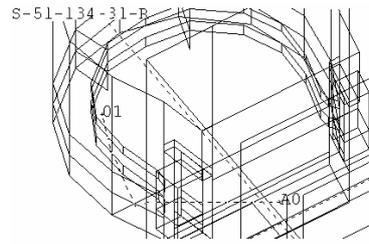
However, to visualise the observed focusing effect, we need to divide the sidewalls into many small surfaces, to show the direction of the focusing "phantom" observed in the Munich Opera.
