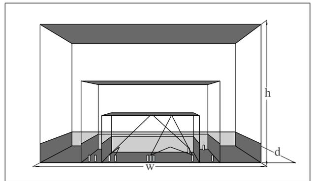
Figure 1. Three stage scenarios with minimum, average and maximum stage size. The source and receiver positions are represented by white columns of 1 m height.
