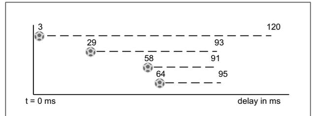
Figure 3. Arrival of direct sound (marked by source symbols and number) and time interval of possible arriving 1st order reflections up to its maximum (dashed lines and number) from self and 3 others, relative to the time of emissions at S-R distance of 1 m on position 'front side' on an average sized stage for synchronized sources.
