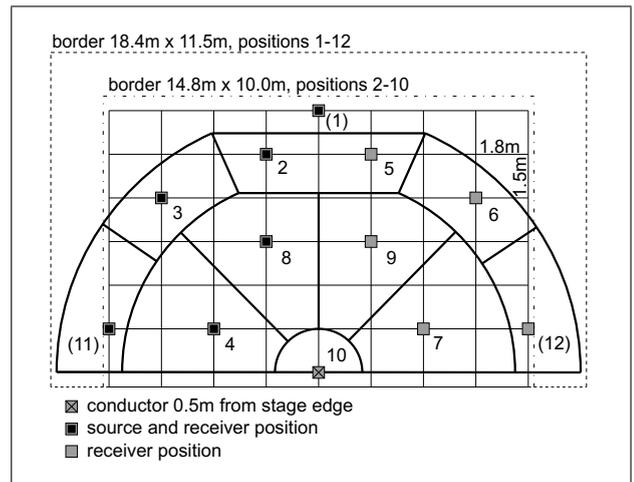
Figure 4. Measurement positions layout.
