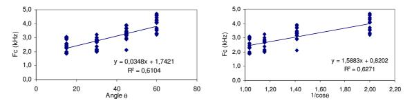
Figure 3. High pass filter cut off frequencies  $F_c$  plotted against incidence angles (left), and against projected element density  $1/\cos\theta$ , re 1 at normal incidence.
