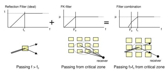
Figure 1. Serial combination of two filters
