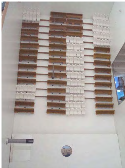
Figure 5. Overhead view of the lecture theatre model with a raked floor and model seating/people. On the right is a viewing window. The disc on stage is the spark source, to the left of the source is a temperature/humidity probe (used for correction for air absorption). In the 6 th row, left of centre, is the raised reference microphone.
