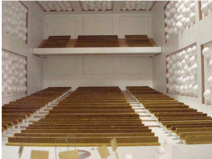
Figure 2. Interior of the 1:25 concert hall with most surfaces with scattering panels. The balcony was omitted for the measurements reported.
