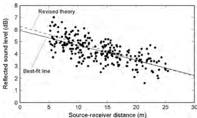
FIG. 5. Measured reflected sound levels in the 500 Hz octave in a model diffuse space, as a function of source-receiver distance [after Chiles and Barron (Ref. 9)].
