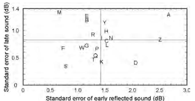
FIG. 7. The SEs for 21 individual halls for early reflected sound plotted against late sound for the 1 kHz octave. The errors in each case are the result of correlation for each hall with source-receiver distance. The hall letters are listed in Table I. The vertical and horizontal lines represent the mean values of the relevant SE.
