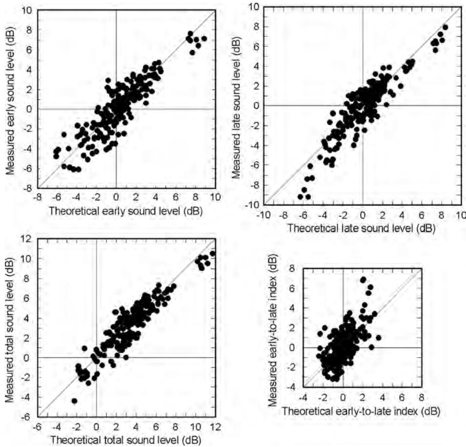
FIG. 4. Measured early, late, and total levels plus early-to-late indices plotted against revised theoretical values for 212 results from 19 concert spaces. Values are the means of the 500, 1000, and 2000 Hz octaves. Diagonal lines represent identity.
