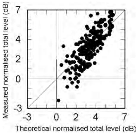
FIG. 6. Measured normalized total levels plotted against revised theoretical values for 212 results from 19 concert spaces. Values are the means of the 500, 1000, and 2000 Hz octaves. The diagonal line represents identity.
