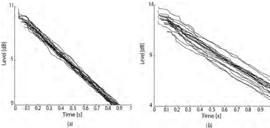
FIG. 3. Integrated impulse decays measured at different locations in a room, plotted with the true onset time relative to the impulse leaving the source. (a) In a diffuse space and (b) in a less diffuse space [after Green (Ref. 30)].
