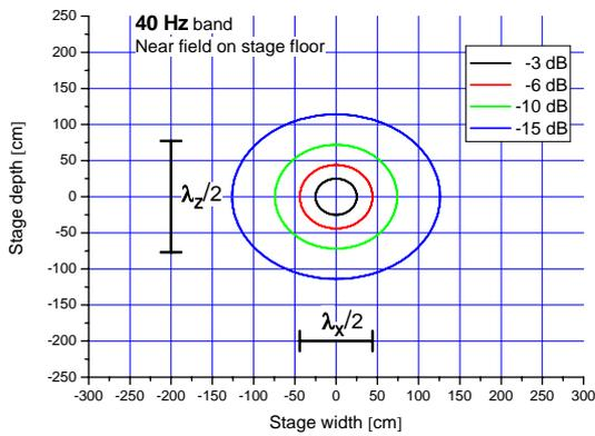
Figure 5. Amplitude distribution at the 40 Hz band.
