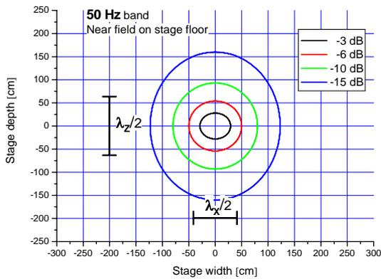
Figure 6. Amplitude distribution at the 50 Hz band.
