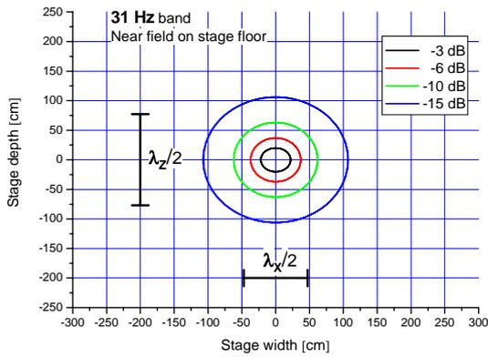
Figure 4. Amplitude distribution at the 31 Hz band.
