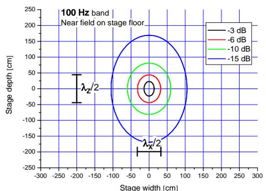
Figure 9. Amplitude distribution at the 100 Hz band.
