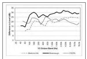
Figure 6. Measured Reverberant Field Noise Reduction between the plenum and the orchestra level.
