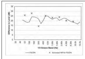
Figure 9. Calculated (X) and measured (–) Reverberant Field Noise Reduction at the Four Seasons Centre for the Performing Arts.
