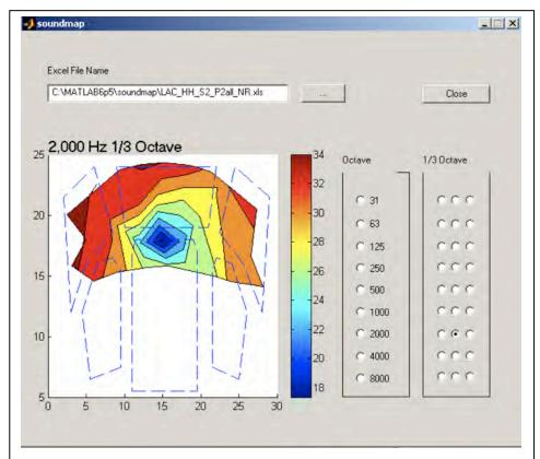
Figure 5. Contour map of Near Field Noise Reduction measurements at the Mississauga Living Arts Centre. The dashed lines indicate the location of seats and aisles on the orchestra level.
