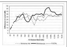
Figure 4. Measured Near Field Noise Reduction between the underside of a slab hole and ear level in the seat directly above.
