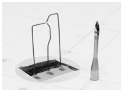
Figure 4.4: Scale model spark source and microphone, 1 m apart.
