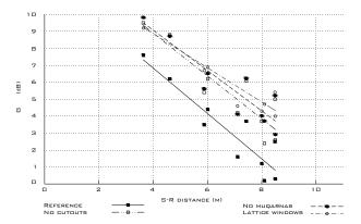
Figure 8: Simulated average strength over the 250-4000Hz frequencies in 4 different configurations
