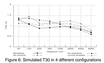
Reference model especially Lattice windows configuration which has increased T30 up to 1.47s.
