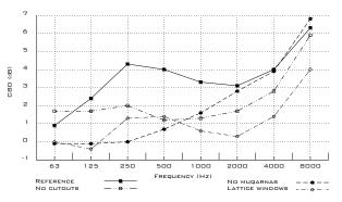
Figure 7: Simulated C80 in 4 different configurations
