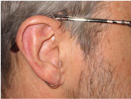
Figure 2: Binaural system for recording the sound pressure at the eardrum. The microphones are behind the pinna, with a hard tube into the ear canal, equipped with a very soft silicone tip. When high quality on-ear headphones are equalized with the same microphones and a mathematical inverse filter exceptional realism results – without the need of head tracking.
