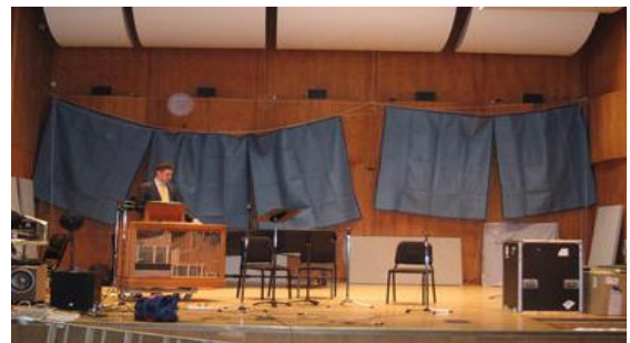
Figure 7: The same hall with some absorption added to the back of the stage.
