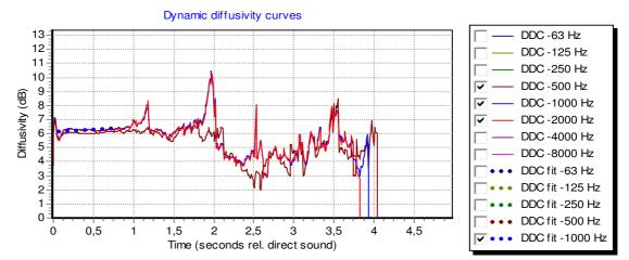
**Figure 1.** A simulated DDC for a room with high scattering coefficients of 0.5 and uneven distribution of absorption (10% on walls and 80% on floor and ceiling). The abscissa is given in time (seconds). Fitted line (blue) shows the best fit for the DDC between -5 and – 35 dB at 1000 Hz.
