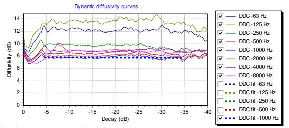
**Figure 6.** DDC at 1000 Hz in the Black Diamond when scattering surface finish has been added to the side reflectors. DDC appears to be quite smooth in the range between -5 and -35 dB and the fitted slope is 0.001 dB/dB decay.  $D_{ss}$ = 8.2 Initial peak= 8.2 dB and the Plateau level is 7.7 dB.
