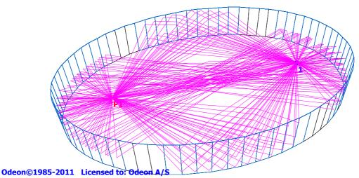
**Figure 7.** Elliptical room with dimensions  $(l \times b \times h) = (30, 20, 4)$  metres. All surfaces are smooth with just 1% scattering. Ceiling and floor are 80% absorbing and walls consists of concrete. Direct sound path, first and second order reflections are displayed.
