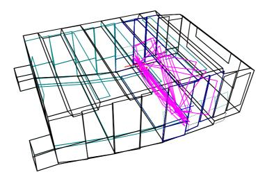
**Figure 4.** ODEON model of the Queens Hall, the Royal Library, Copenhagen. Reflections repeats continuously between four reflector panels that is tilted slightly towards each other – creating a flutter echo when reflector panels are left without any scattering surface finish.
