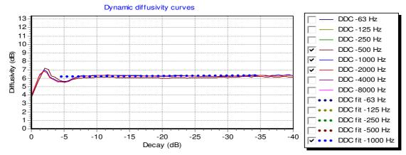
**Figure 2.** DDC for a room with high scattering coefficients of 0.5 and uneven distribution of absorption (10% on walls and a 80% on ceiling). The abscissa is given in Decay (dB). Fitted line (blue) shows the best fit for the DDC between -5 and – 35 dB at 1000 Hz.
