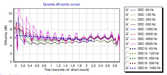
**Figure 8.** DDC for impulse response in the focus point of the elliptical room displays strong ripples.  $D_{ss}$ =8.5, Initial peak = 9.7 dB, plateau level= 6.7 dB. Note that abscissa is in time (seconds), giving a clearer view of the echo (frequency bands are time aligned and time between strong reflections is equidistant.
