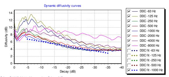
**Figure 5.** DCC in model of the Black Diamond when side reflectors are without scattering surface finish. DDC has pronounced ripples in the range between -5 and -35 dB and the fitted slope is 0.13 dB/dB decay (drops 3.9 dB over 30 dB).  $D_{ss}$ = 8.3 dB. Initial peak= 8.0 dB and plateau level is 4.7 dB.
