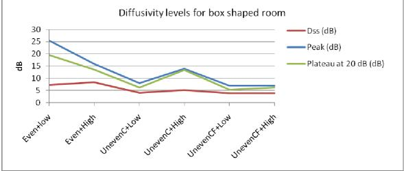
**Figure 3.** Diffusivity levels extracted from DDC at 1000 Hz. Even/Uneven refer to the distribution of absorption (UnevenC with absorption on ceiling and UnevenCF with absorption on ceiling and floor) – low and high refer to the amount of scattering.
