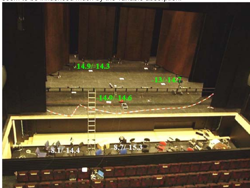
Figure 31: Stage support ST_{Early}/ST_{Late} [dB]. Elements from the orchestra shell were used on the stage as a set.
