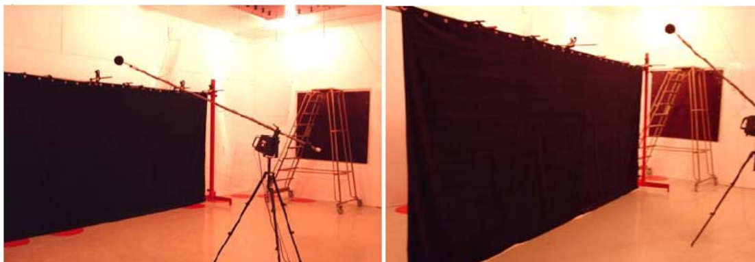
Figure 13: Reverberation lab measurements at SINTEF 'Byggforsk' Oslo. Left: Drape hung 250mm from wall. Right: Same drape 'freely suspended'. [Photo: Anders Buen]
