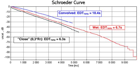
Figure 5: Example of a close (d=0.3\*reverberation radius, Rr) recorded IR (black) convolved with a wet IR (red) making the convolved (blue) IR.
